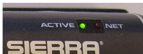
Figure 7 LED's showing the activities of the Compod
