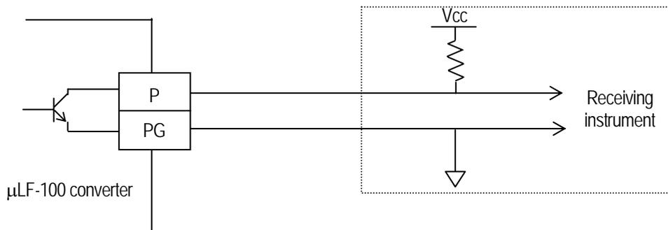
◆ Example of connecting the integrated reset signal input
