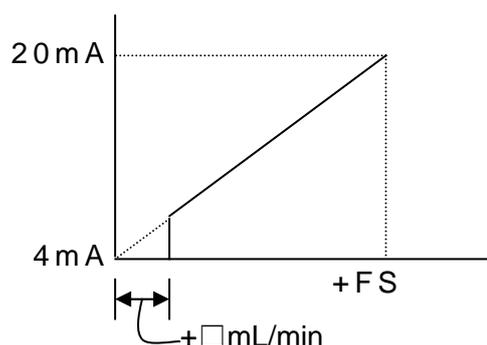
A flow rate output of □□□□.□□ mL/min or lower is regarded as 4 mA.
