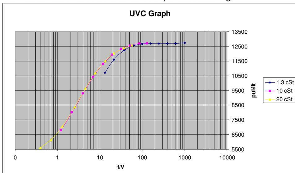
The blue line (=1,3cSt or mm<sup>2</sup>/s) shows the limitations of the UVC method. It can be seen that at least 3 points deviate significantly from the ideal UVC line. These outlying calibration points will not be used for linearization and temperature compensation.
