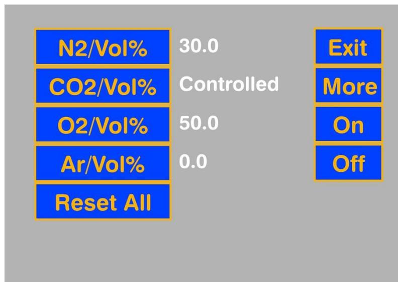
When the gas mixer function is selected, the first 2 - 4 registered MFCs (see: Registration of MFCs) are combined into one mixer.
