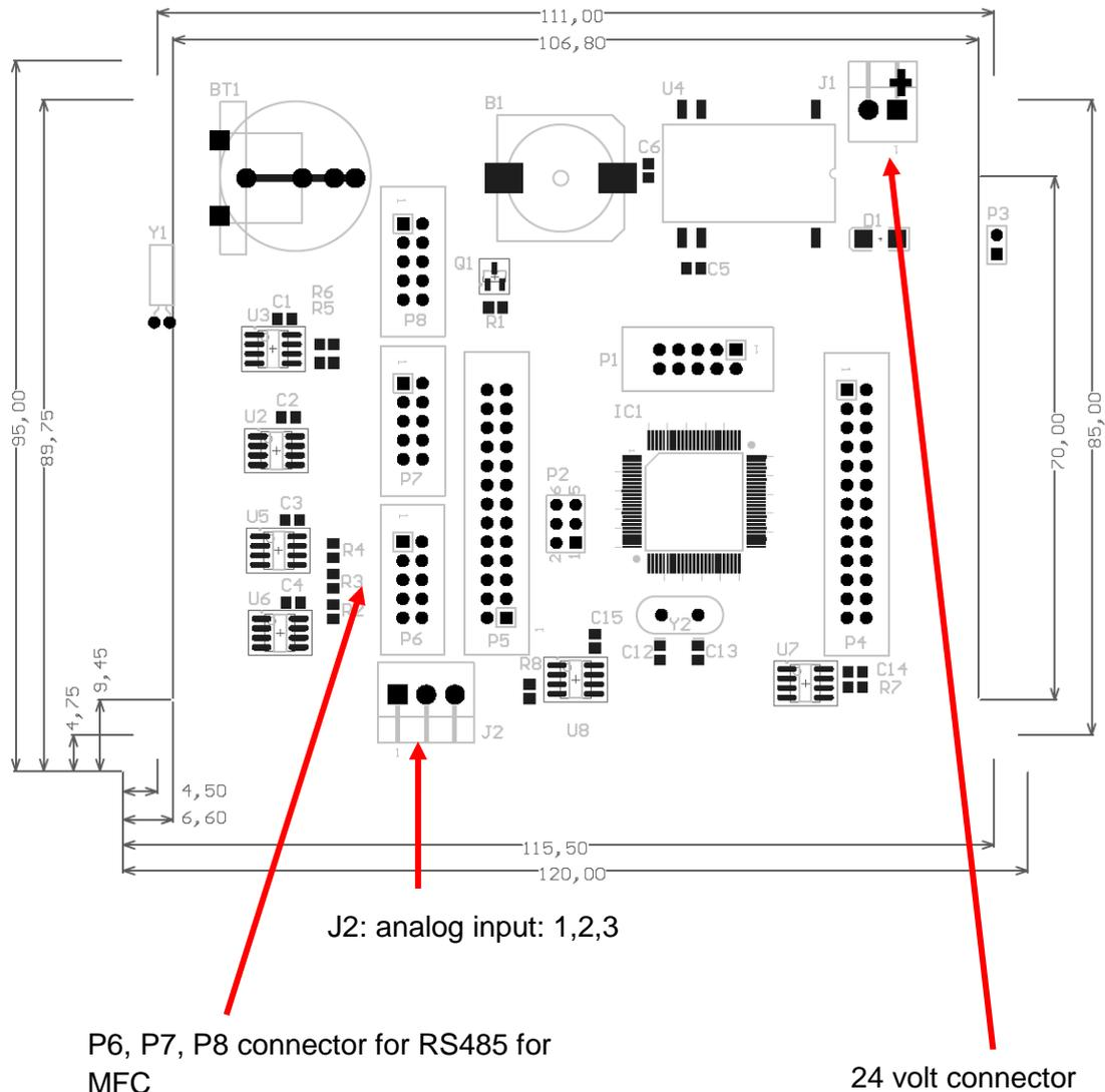
Connector sockets on the display pcb:
