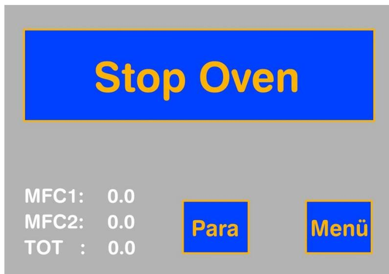
Now the oven can be switched off at any time by pressing the Stop button. It will likewise be immediately switched off if the system detects a bad condition.
