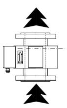
A straight run of pipe (without valves, curves, etc.) with a minimum length of five diameters up and three down stream of the flow meter should be maintained.
