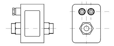
Body and end connection material is 316 stainless steel with optional material available.
