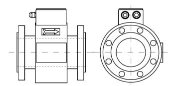
Body and end connection material is acrylic painted carbon steel with optional material available. End connections are ANSI flange with additional options.
